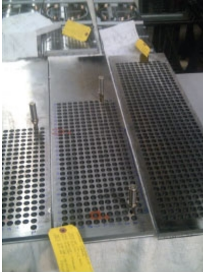
In a tooling test, a manufacturer drilled holes in 4140 stainless steel with a Mazak CNC until the tool failed. Using standard fluid, machinists were able to cut 20 rows of holes. Using Tool-X coolant, machinists ran out of space on the plate after 42 rows of holes without a failure.
