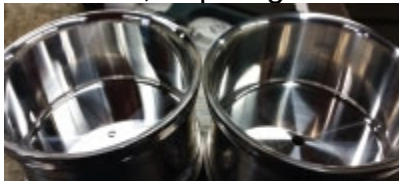
Aluminum wheels machined with Tool-X's 703 coolant (left) had higher output rates than those machined with traditional fluids (right), and the manufacturer was able to eliminate a polishing step.
