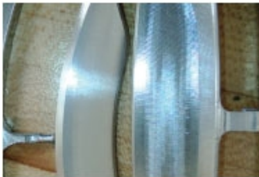
Prototype aluminum wheels, machined on CNC turning centers, experienced better surface finishes and higher speeds and feeds when the manufacturer switched cutting coolant.
